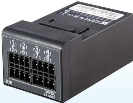
The MOD-IO8 is an 8 channel I/O module that fits into any modular controller.
