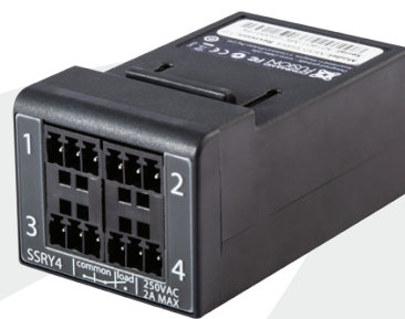
MOD-SSRY4 Solid-state relay module 4 x 250VAC 2A non-latching normally-open solid-state relays
